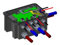
17. The Silicone applies inside the main housing around
